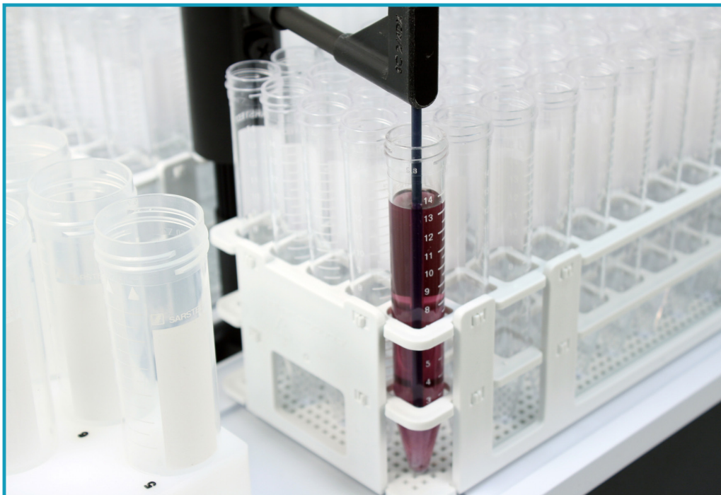
Figure 6. Simply pour solution (syrup) into tube and start analysis. Sample is autodiluted inline to appropriate TDS.
